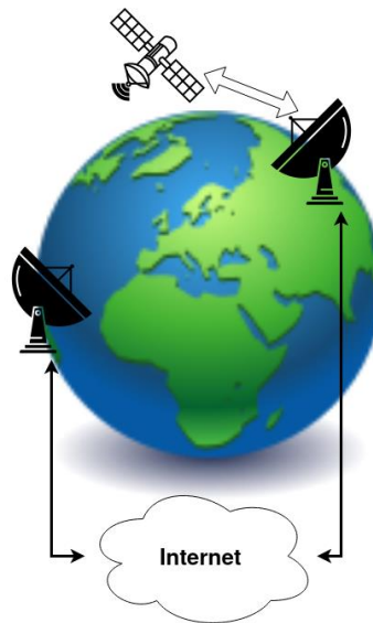
Figure 6.20: SatNOGS multiple ground stations connected through the internet
