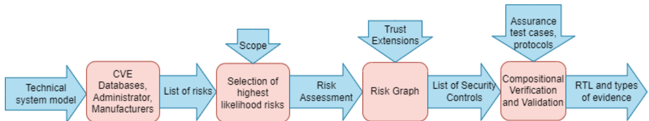
Figure 4.2: REWIRE threat modelling pipeline
